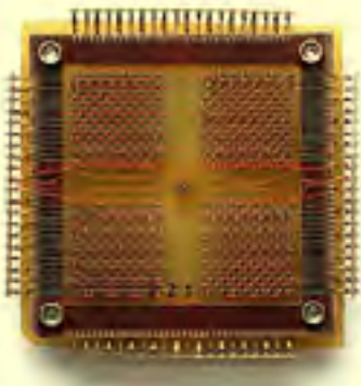
Core memory, the RAM of its day. Source: Wikipedia
