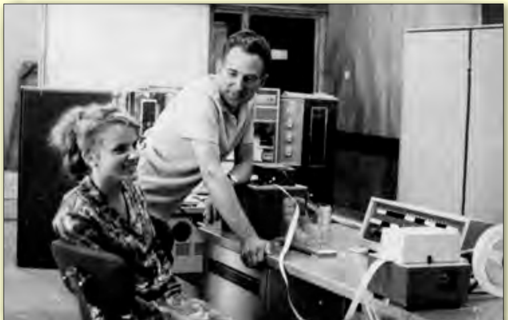
Operators running Final Acceptance tests on ZAM-41.
