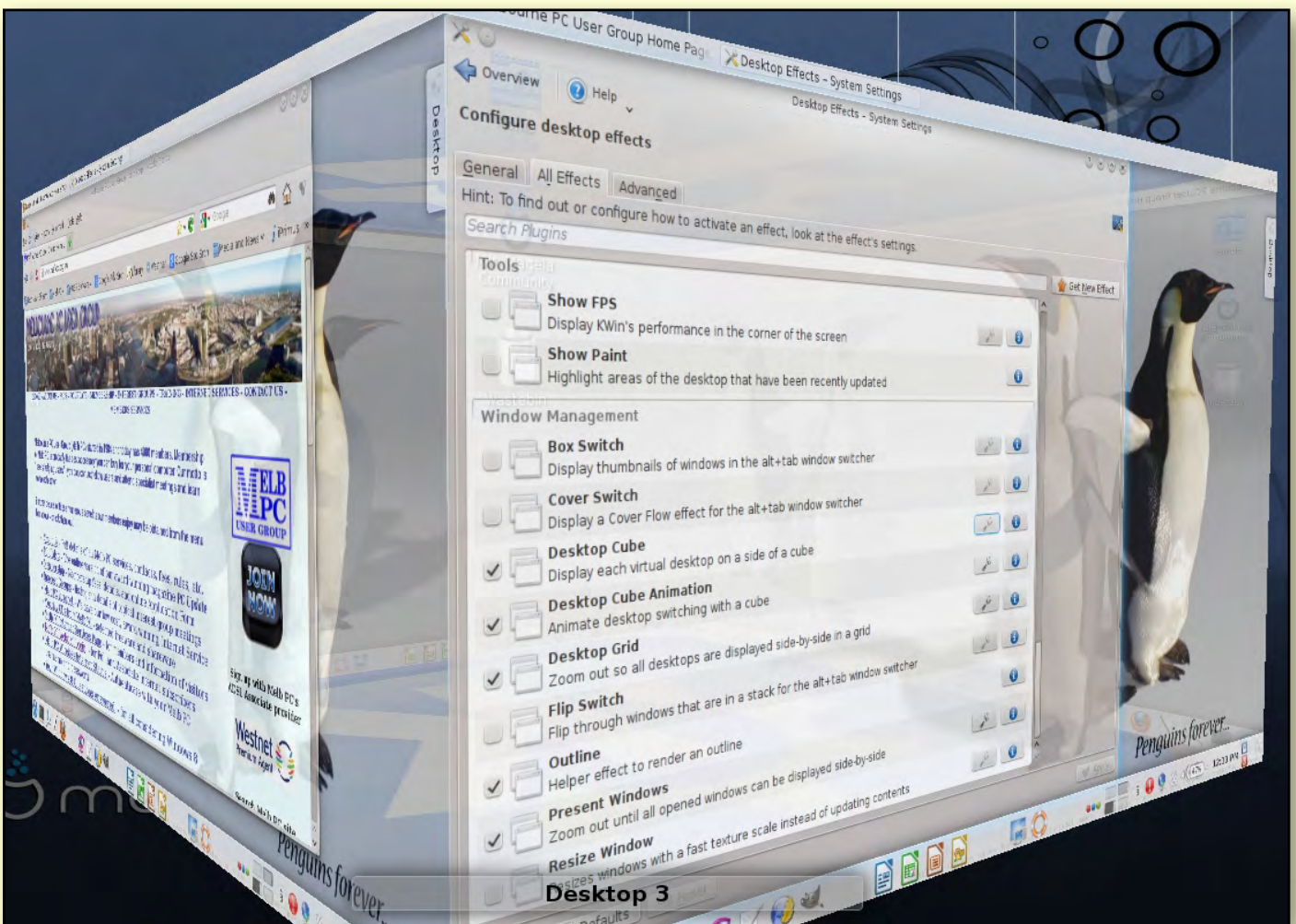
Figure 2. The KDE cube – to switch desktop workspaces, use the mouse scroll wheel to rotate the cube until the desired desktop is shown. Alternatively, use CTRL/F11 and then left-click to rotate or tilt as needed: right-click to select a workspace.
