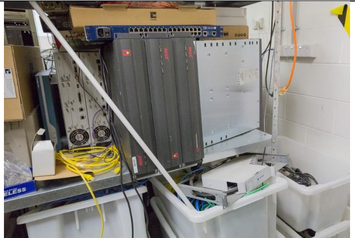
Suite 3B, Spares rack, Decommissioned Ascend & Portmaster, from dial-up days. Remote Access Servers.
