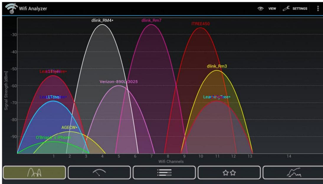
Figure 3 – WiFi Analyser Channel & Signal Strength graph
