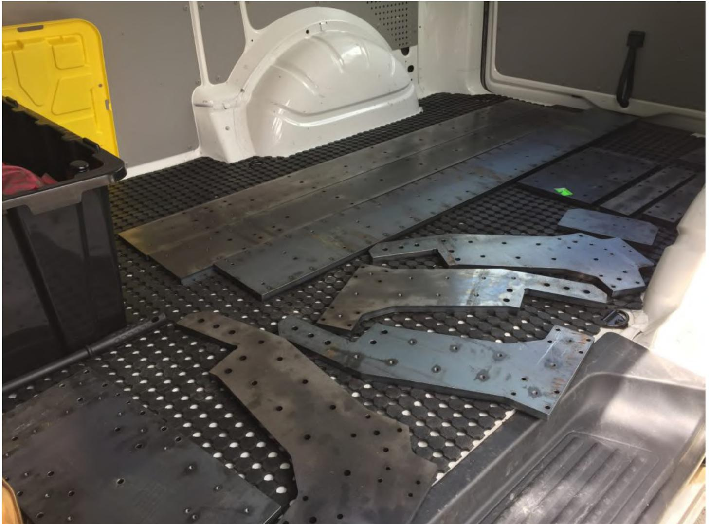
The laser cutting worked rather well, it's quite a clean-cut edge compared to the plasma cutting that I was initially considering.
