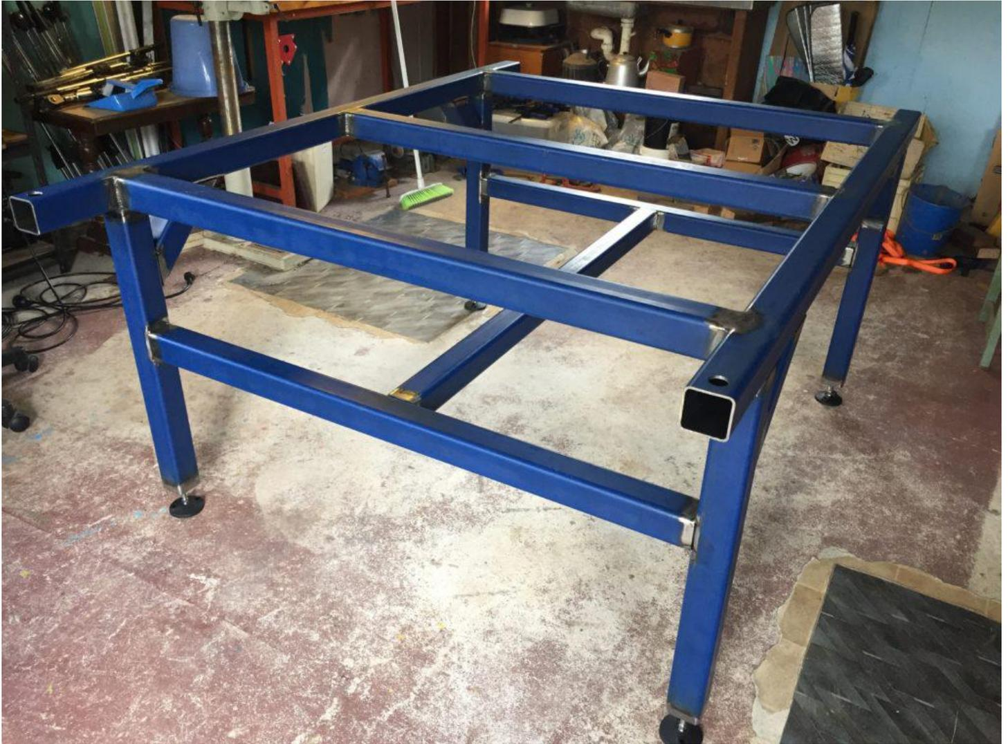
It was a couple of weeks until I was able to do a second lot of welding, but I was able to get all joins finally welded up. It's nice and heavy and solid, and should serve as a good base for the machine!
