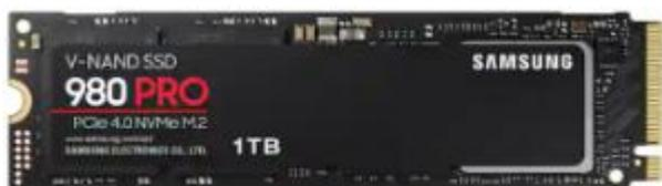
The second new form factor is called NVME (Non-volatile Memory Express). An NVME SSD does not include a SATA controller; it is directly connected to the PCIe data bus of the motherboard via a simple memory controller interface. The NVME SSD card also plugs into an M.2 socket on the motherboard. The NVME SSD card only has a single notch (M only) in the connector end.
