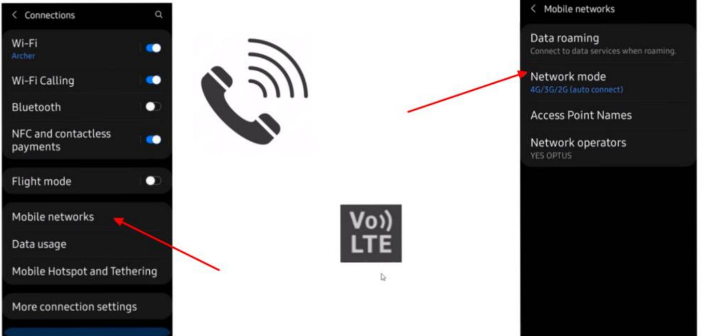
Figure 9 - Enabling VoLTE on the Samsung A20 (Screen capture from Stewart's presentation)
