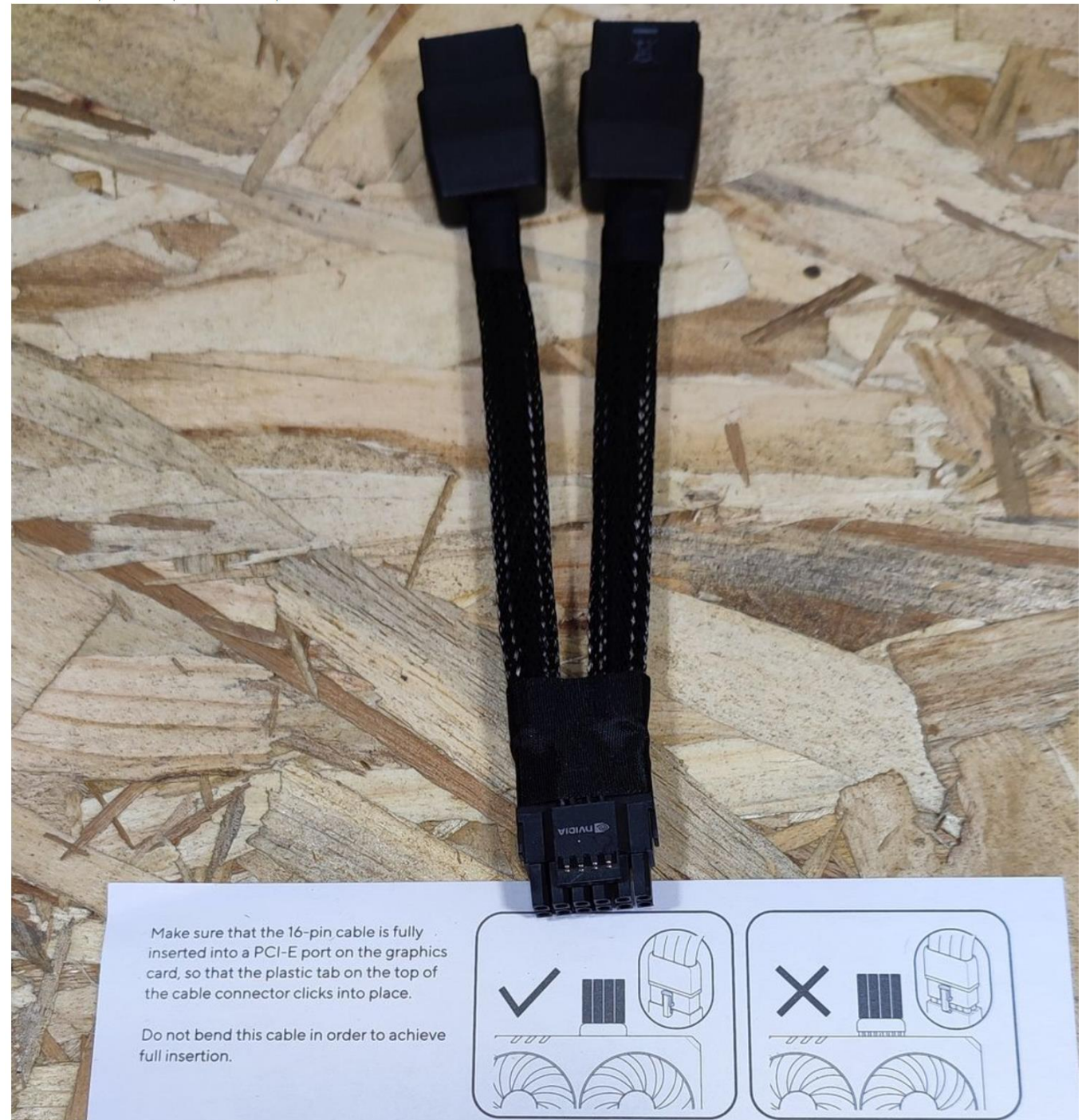
The dual 8-pin to 16-pin cable adapter:
