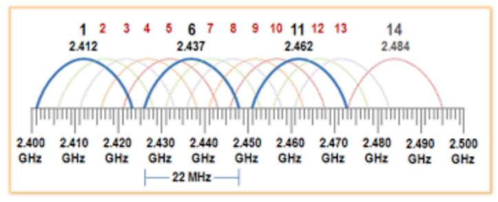
This diagram shows the frequency and channel distribution for 2.4GHz. Rob/Stack Exchange, CC BY-SA
