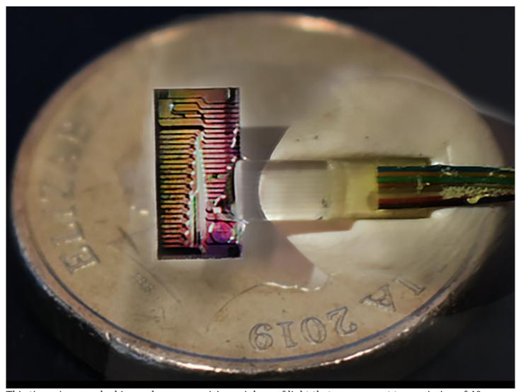
This tiny micro-comb chip produces a precision rainbow of light that can support transmission of 40 terabits of data per second in standard optic fibres.
